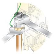
Feed cable into Case. Fit Earth sleeve (not supplied) and then strip insulation.
