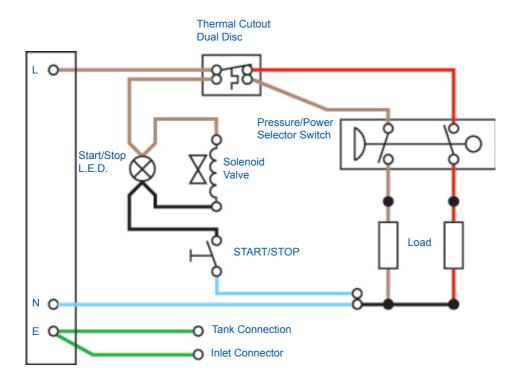
**Internal Wiring Diagram**
